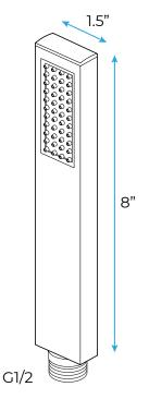
Flow Rate: 2.0 GPM / 7.6 LPM
